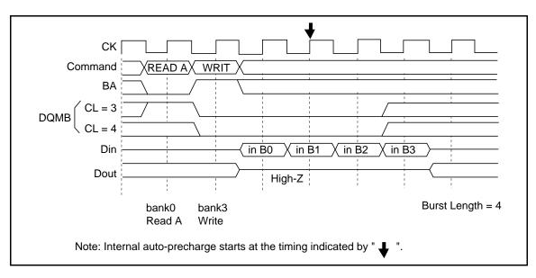
**Read with Auto Precharge to Write Command Interval** (Different bank)
