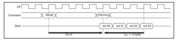
READ to PRECHARGE Command Interval (same bank): To stop output data
