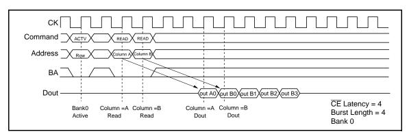
**2.** Same bank, different ROW address: When the ROW address changes on same bank, consecutive read commands cannot be executed; it is necessary to separate the two read commands with a precharge command and a bank-active command.
