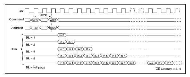
**2. Single write:** A single write operation is enabled by setting OPCODE (A9, A8) to (1, 0). In a single write operation, data is only written to the column address and the bank select address (BA) specified by the write command set cycle without regard to the burst length setting. (The latency of data input is 1 clock).
